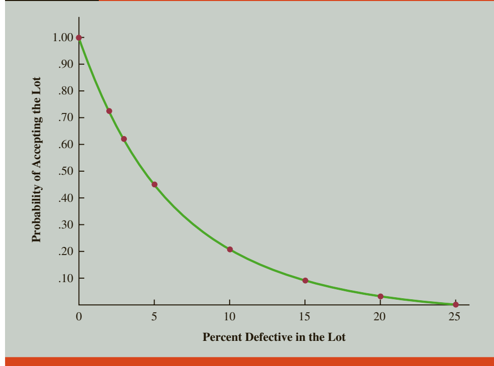
FIGURE 21.12 Operating Characteristic Curve for the n = 15 , c = 0 Acceptance Sampling Plan
