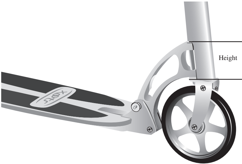
FIGURE 7.4 Rendering of a Xootr Scooter, Including Its Steer Support Component
