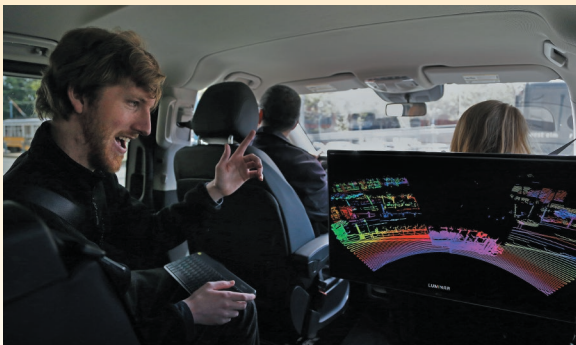
This is the digital image taken from the Luminar Lidar. Volvo plans to offer the system in driver-assisted vehicles equipped with the “Lidar and perception stack.”
