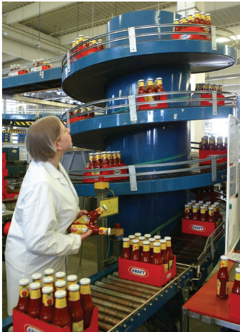
HERE A WORKER VISUALLY CHECKS CARTONS OF KETCHUP AS THEY MOVE ON A SPIRAL CONVEYOR AND REPLACES BOTTLES THAT ARE NOT PERFECT. THIS PROCESS COULD PROBABLY BE MADE MORE EFFICIENT.
